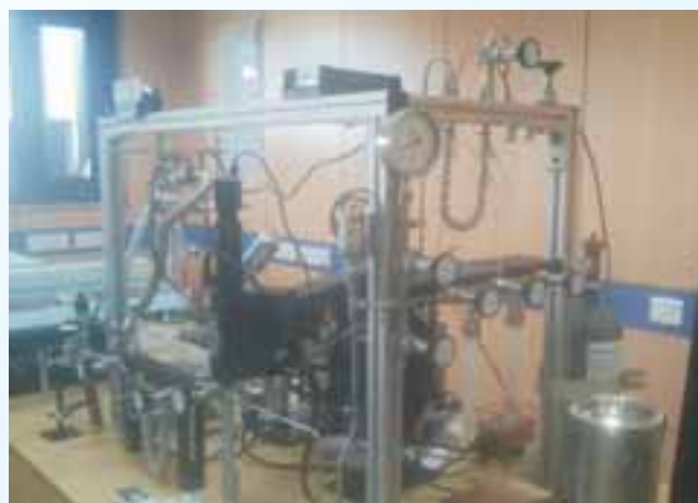
Fig. 12: \text{BrF}_5 Laser Fluorination System for measurement of \delta^{18}\text{O} in silicate minerals, established at WIHG.
