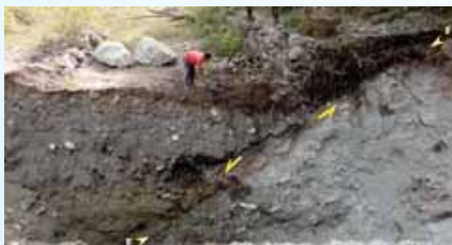
Fig. 25: A part of the trench wall across Logar Gad fault (F-F) at Logar village in the vicinity of the MBT in Kumaun Himalaya. Reactivation after giant earthquakes on the mega thrust is considered to generate this normal fault.
