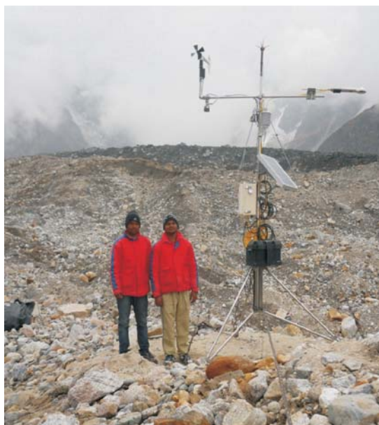
Portable Automatic Weather Station installed at the Chorabari Glacier surface (3930 m a.s.l.). The station is equipped with the sensors of air temperature, relative humidity, surface temperature, wind speed and direction, atmospheric pressure, snow accumulation, incoming & outgoing both shortwave and long wave radiations.
