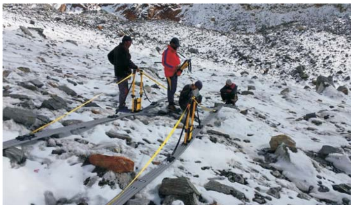
Installing an instrument to monitor atmospheric black carbon in Gangotri Valley, Garhwal Himalaya.
