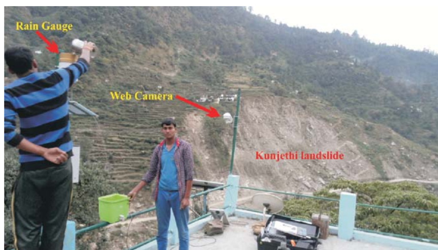
View of the Landslide Monitoring System comprising web camera and rain gauge installed on the right bank of the Kali valley, opposite Kunjethi village.
