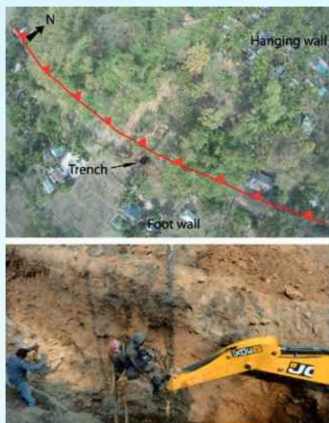
Fig. 77: The top image is the bird's eye view of the fault scarp with an excavated trench location at the base of the scarp. The photograph was taken using the Ricoh GR digital camera, which was mounted on a DJI Phantom I unmanned aerial vehicle. The bottom left portion shows farmed flatland (footwall), and the top right portion is the uplifted fault scarp (forest and village area) (hanging wall). The bottom image is the view from the ground surface of the trench, carrying out scraping of the walls and collecting charcoal samples.
