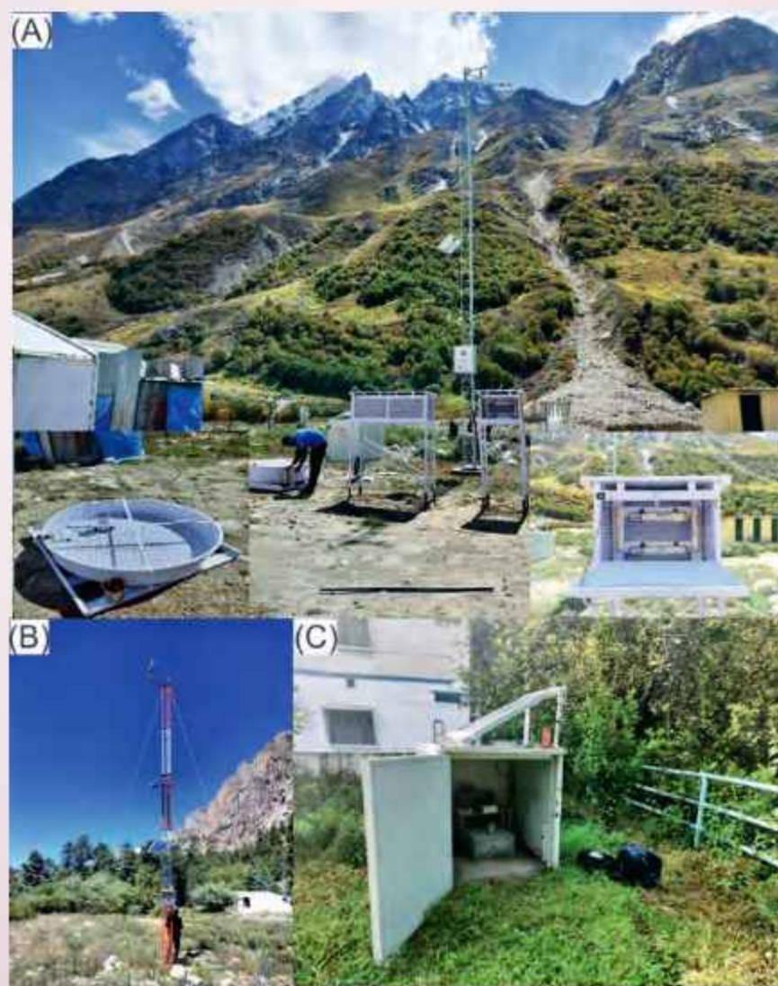
Fig. 95: (A) Photograph showing the observatory at the base camp, equipped with an Automatic Weather Station, Broadband Seismic Station, and manual instruments such as maximum-minimum thermometers, an ordinary rain gauge, and a pan evaporimeter installed in September 2024. (B) The Automatic Weather Station at Chirwasa and (C) the Broadband Seismic Station at Maneri.
