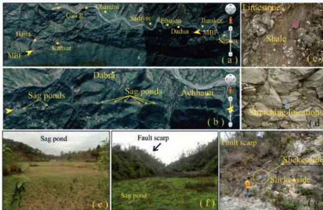
Fig. 51: (a) Google Earth images showing fault trace of the Main Boundary Fault (MBF) between Sataun and Baila (marked by yellow triangles), the fault scarp is south dipping with development of sag ponds along the fault trace; (b) Google Earth image showing sag ponds in a linear arrangement along the fault trace; (c,d) highly sheared bedrock and stretching lineation observed in the footwall block of the MBF; (e,f) formation of sag ponds on the downthrown side of the fault; (g) south dipping fault scarp showing slickensides in the bedding planes indicating bedding parallel movement in the limestone.
