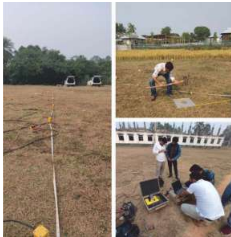
Fig. 2a. MASW field set up.
